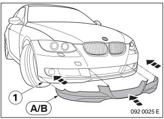
Carefully place front attachment **A/B** onto the bumper (1) and position exactly.
