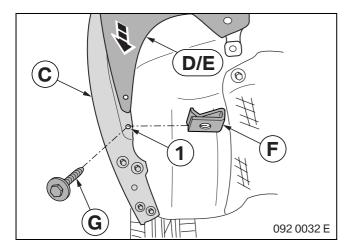
To mount exhaust cover **D/E**, attach sheet nut **F** to bumper **C** and affix with bolts **G**.
