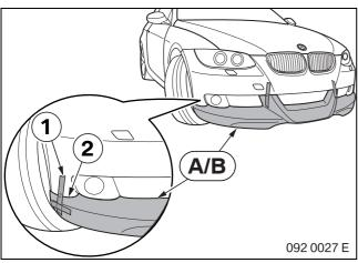
Press all over front attachment **A/B** to ensure attachment and protect against slipping with tape (1).
