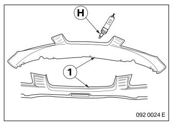
Apply adhesive **H** evenly to the gluing surfaces (1) **on the inside**.
