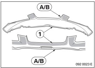
Roughen glue surfaces (1) **on the inside** of front attachment **A/B** with the sandpaper included in the adhesive kit and then clean with Betaclean.
