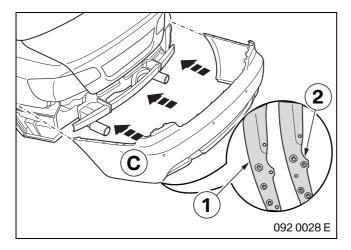
Mount rear bumper **C** on the car according to TIS. In 4/6 cylinder cars, bumper **C** is affixed with 3 bolts (1). In Turbo cars, bumper **C** is affixed with 4 bolts (2).
