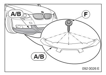
Affix front attachment **A/B** at the five screw fastening points with bolts **F**.
