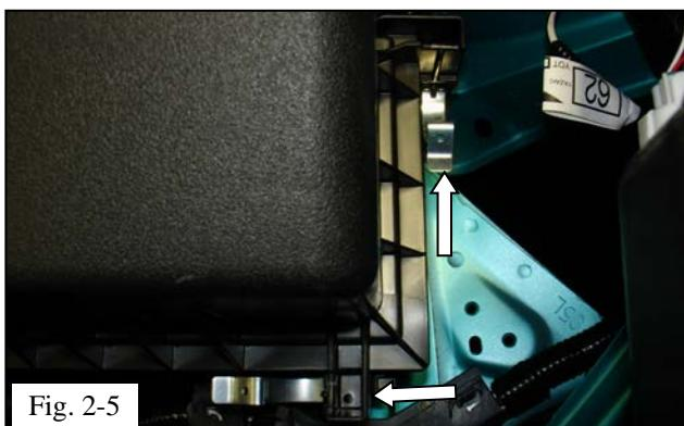
(e) Unclip the two air box clips (Fig. 2-5).
