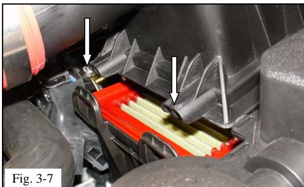
(g) Guide the inboard mounts of the air box top into the loops on the OEM lower air box (Fig. 3-7).
