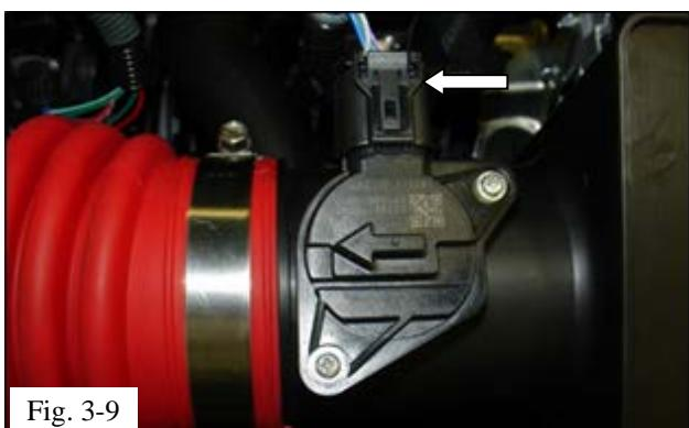
(i) Plug in the mass airflow sensor connector and secure the wire harness to the airbox (Fig. 3-9).
