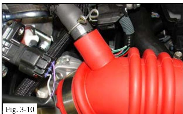
(j) Reconnect the crankcase vent hose to the TRD air intake bellows. Secure the assembly with a spring clip (Fig. 3-10).
