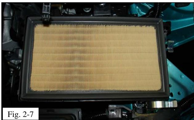
(g) Remove the OEM air filter (Fig. 2-7).
