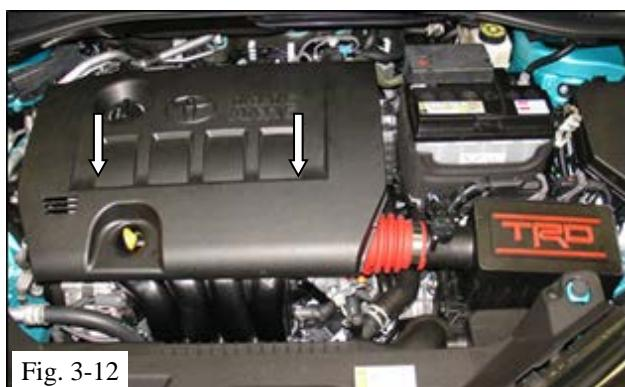
(l) Reinstall the engine cover by aligning engine cover grommets above mounting pins and push down to install the engine cover (Fig. 3-12).
