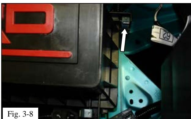
(h) Ensure that the upper airbox is properly seated on the air filter and secure the upper air box with the 2 air box clips (Fig. 3-8).
