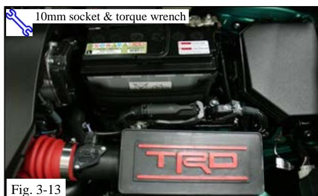
(m) Do a final check to ensure all wires and hoses are secure. Reconnect the negative battery cable to the negative battery terminal (Fig. 3-13).
