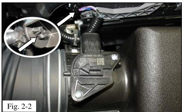
(b) Unplug the MAF sensor and unclip the MAF sensor wiring harness from the OEM air box lid (Fig. 2-2).
