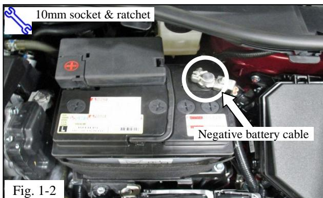
(i) Remove the negative battery cable (Fig. 1-2).
