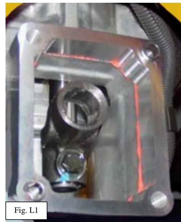
→ 3. Install shift lever retainer on to spacer. Again, make sure dowels engage correct larger counter-bored holes.
