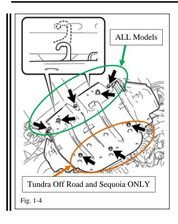
(d) Remove the 3 screws and 5 bolts (Tundra Off Road and all Sequoia models) or the 3 screws and 2 bolts (other Tundra models) attaching the OE engine undercover. Unhook the cover as shown (Fig. 1-4). Discard the OE cover, bolts, and screws.
