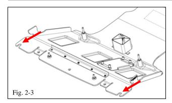
(c) Align the forward edge slots of the skid plate (red arrows, Fig. 2-3) with the two tow hook fasteners that were partially threaded in Step 1(c).
