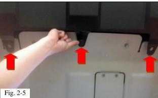
CAUTION: Ensure the front bumper plastic tabs are on the outside of the skid plate (three places); do not secure them at this time (Fig. 2-5).
