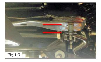
(c) Temporarly install the front most tow hook bolts, leaving an approximately 1/2" gap between the bolt washer face and the underside of the frame (Fig. 1-3).
