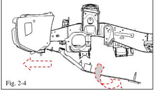
(d) Push the plate forward and rotate the rear section up, ensuring the rear fasteners go through the holes in the center member bottom and the top holes (Fig. 2-4).
