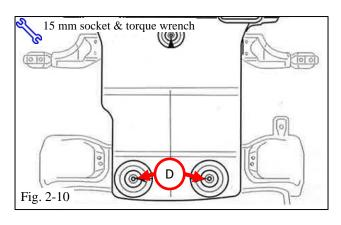
(2) The smooth face of the angled wedge washers should be contacting the nut. The counter-bored hole face of the angled wedge washers should be contacting the top surface of the frame crossmember.
