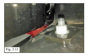
(a) Check the angled washer orientation on the cross member to ensure the thickest side of the washer remains facing toward the center of the vehicle (Fig. 2-11).
