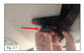
(f) Locate the plastic ratchet fasteners and install them through the plastic bumper tabs into the holes on the skidplate (3 places) (Fig. 2-5 & Fig. 2-7).
