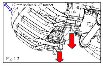
(b) Use a ½" ratchet and 17mm socket to remove the tow hooks. Save them for reinstallation (Fig.1-2).
